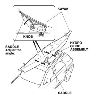
Slide the kayak forward or backward until it's level with the roof. If necessary, loosen the knob on each saddle and adjust the saddle angle to fit snugly against the kayak. Tighten each knob securely. 6. Route each strap with buckle through a buckle cover with the ribbed side facing up.
