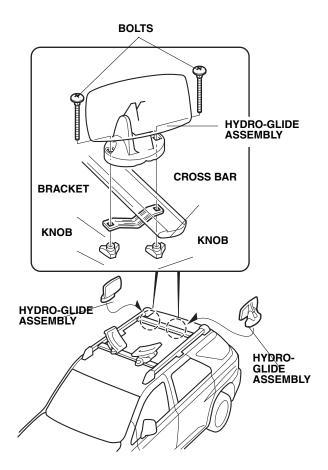
3. Set the front of the kayak on the hydro-glide assemblies. Standing behind or alongside the kayak, lift up the rear of the kayak and push it forward onto the hydro-glide assemblies and saddles. Make sure the kayak reaches the front saddles before you lower it
