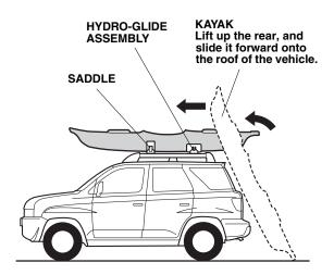
Adjust the distance between the saddles and the hydro-glide assemblies to the same width as the kayak, then secure the saddles and the hydro-glide assemblies by tightening the knobs you installed in steps 1 and 2.
